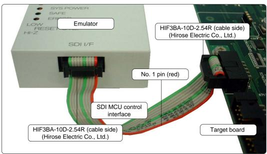
Figure 3.3 Connecting the SDI interface cable
